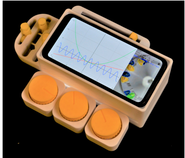
Figure 10: Interactive graph, the buttons are used to select the current function. The dials control the a , b and c parameters of the functions in the graph. The slider is used to zoom in and out on the x -axis.
