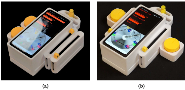
Figure 9: Two designs of the music interface. In both cases the two sliders control the volume and the two dials control the tempo of two separate tracks. The button on top plays/pauses both tracks. The screen shows the camera output and the current parameters of the tracks. The interface on the left (a) groups widgets by functionality whereas the interface on the right (b) groups widgets by track.
