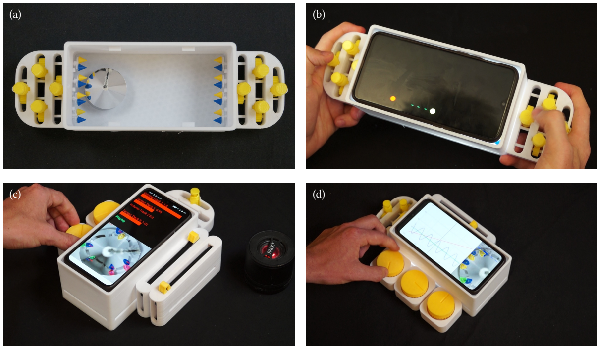
Figure 1: ClipWidgets are interactive widgets attachable to a dedicated phone case. Markers on the widgets are reflected on a conical mirror in the phone case that makes them visible for the phone camera when inserted (a). We demonstrate three applications of ClipWidgets: a game controller (b); a music-mixing interface (c), and a mathematical equation explorer (d).
