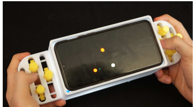
Figure 8: Game controller prototype consisting of two sets of four attachable buttons. The left four buttons are used to control the position of the player (white dot on the screen), and the right four buttons are used to shoot enemies (orange dots) in four directions.
