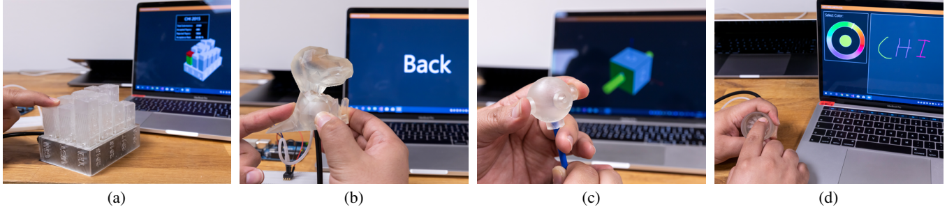
Figure 8: Example AirTouch Applications. With AirTouch, interactive objects are fabricated as a single structure without any post-print assembly or calibration. We showcase objects of different geometries augmented with AirTouch: an interactive bar chart (a); interactive animals (b); grasp-sensing sphere (c); and a color hue selector (d).
