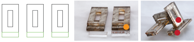
Figure 7: For our conductive layer tests, we cut objects of fixed geometry (left) with varying conductive layers. We clipped them to an ItsyBitsy at the orange point and attempted to use the CapTouch library (centre). We then measured resistance across single parts, and through 1 and 2 joints at, e.g., the two joints between the red points (right).
