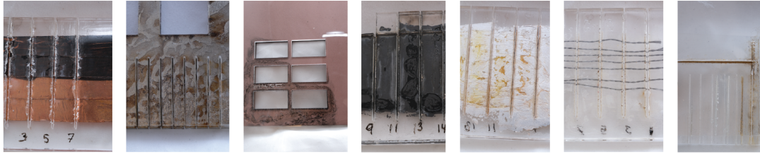
Figure 6: Instances of all conductive materials explored with LaCir, fabricated using acrylic structural layers for visibility (copper tape and darkened copper tape, silver paint, copper paint, carbon paint, silver leaf, conductive thread, ITO). The conductive threads seen here did not work well, so we do not report formal experiments with them.
