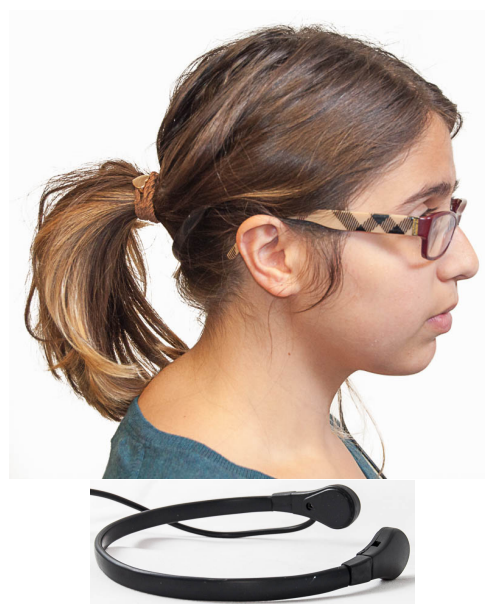
Figure 1. The bone-conduction microphone used in Bitey (bottom) and its nearly invisible positioning on the temporal bone just above the ear (top).
